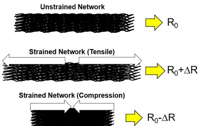
Fig. 4. Schematic of buckypaper before and after being stretched. The induced gaps in the conductive network increases electrical resistance.
