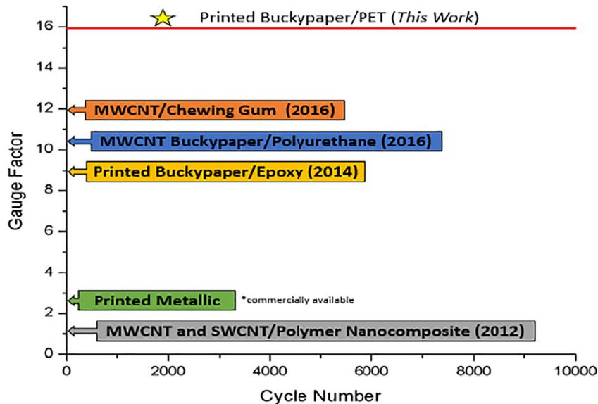
Fig. 7. Comparison of commercial and other CNT-based sensors' gauge factors. The printed BP sensor's gauge factor remains consistent for >10,000 cycles.
