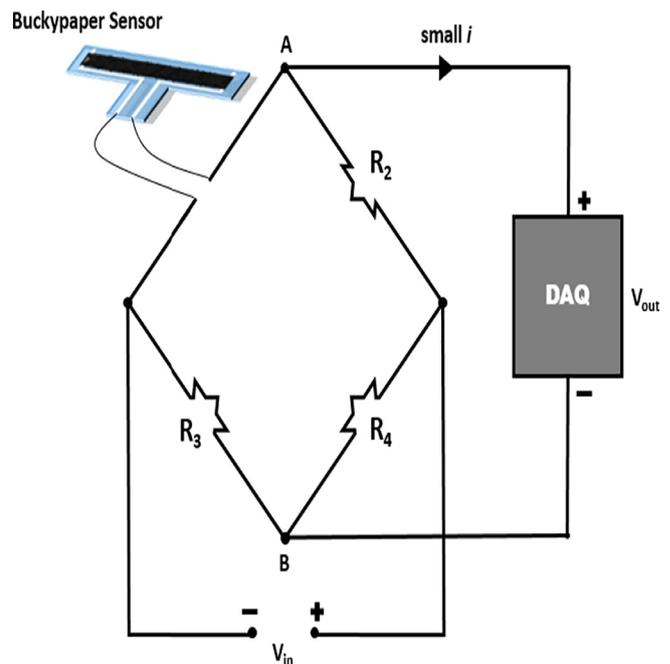
Fig. 5. Schematic of the Wheatstone bridge characterization setup, where  $V_{\text{in}} = 3 \text{ V}$  and  $R_{\text{BP}} \approx R_2 = R_3 = R_4$  to balance the bridge.
