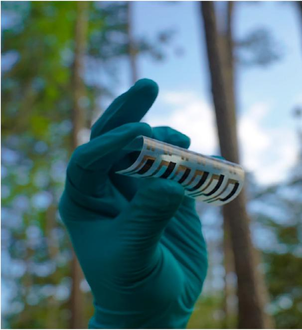
Fig. 3. BP strain sensors offer a low-profile and flexible design.
