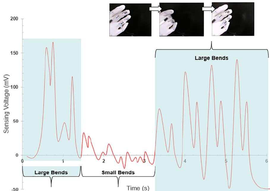
Fig. 8. Experimental results from monitoring fingers using BP strain gauge that was fastened to a glove.
