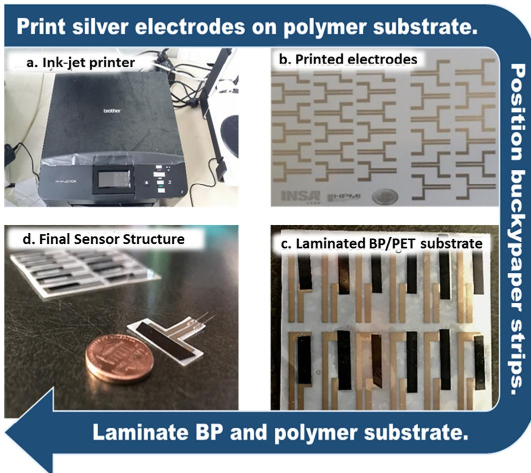
Fig. 2. Manufacturing process flow for buckypaper strain sensors. It includes printing, laminating, and cutting.
