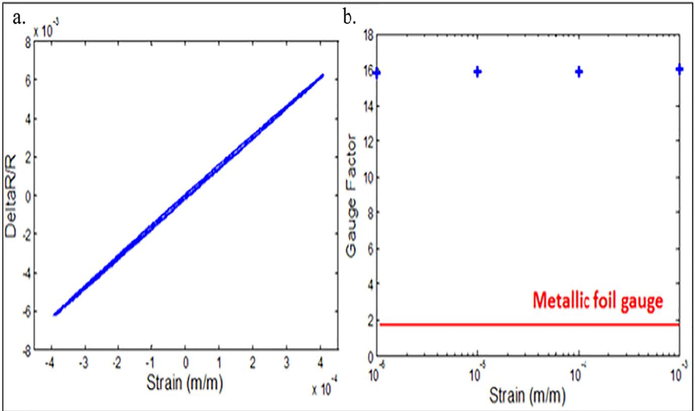
Fig. 6. BP strain sensor's dynamic response: (a) Measured sensitivity based on a Wheatstone bridge configuration. (b) Gauge factor versus strain comparison.
