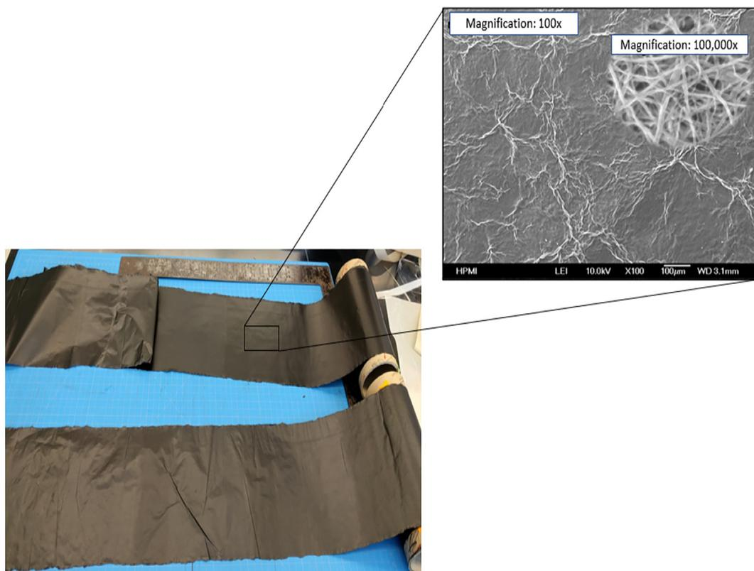
Fig. 1. Multi-wall carbon nanotube buckypaper; a. continuous roll of MWCNT buckypaper, b. scanning electron microscopy images at 100 $\times$  and 100,000 $\times$  magnification.
